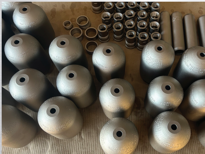
ENP significantly increases the life of carbon and stainless steel parts.
