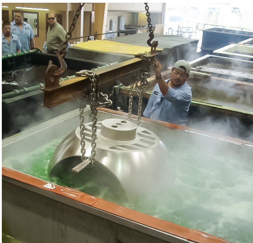
© Houston Plating & Coatings | Electroless Nickel plating provides superior resistance to corrosion and significantly increases the life of carbon and stainless steel parts
